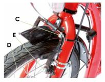
do this, loosen the clamping screw  $(\mathbf{C})$ , press the brake blocks together by hand, pull the Bowden cable taut and then re-tighten the clamping screw. If the brake blocks are not accurately aligned with the rim edge  $(\mathbf{D})$ , you must readjust them accordingly. In order to change the alignment of the brake blocks, loosen the screws  $(\mathbf{E})$ . Leave this work to your specialist dealer in case of any uncertainty.
