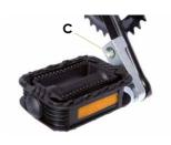
The position of the pedals must be conducted so that the amplitude of the pedal depicts the flexibility of the knee joint. In the lower pedal position, the maximum extension to be achieved, and in the upper position, the maximum flexion of the knee is to be achieved. This adjustment is to be undertaken in interaction with the saddle height. In order to adjust the crank shortener, loosen the pedals with a 15 mm open-end wrench and place it into the opening (**C**).
